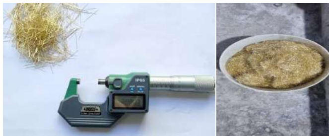
Steel Fibers : length=13 mm, Dia =0.15mm
